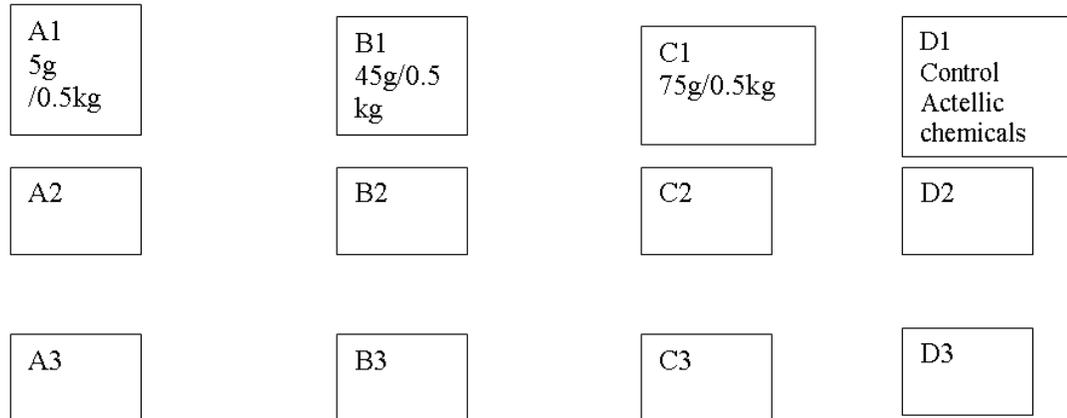
Hessian bags were used for the experiment and were arranged in the manner depicted in Fig 3.1. The room was clean and ventilation was guaranteed to ensure that the weevils had sufficient air supply. In addition, the grain bags also allowed for air movement without allowing them to migrate out of the bags. Blocks indicate replications for each level of ash concentration.
